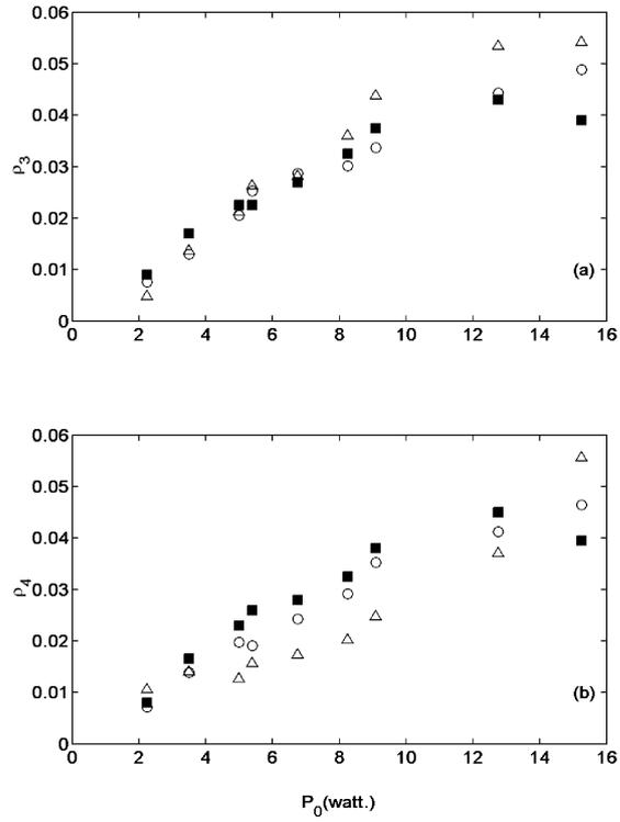
Figure 3.8: Comparison between the experimental measurements (filled squares), simulations without stochastic phase fluctuations (open triangles) and with stochastic phase fluctuations (open circles) of the first-order sideband power versus pump input power for  $L=50.39$  m, and  $\Omega = 366$  GHz: power in the (a) blue-shifted sideband and (b) red-shifted sideband.
