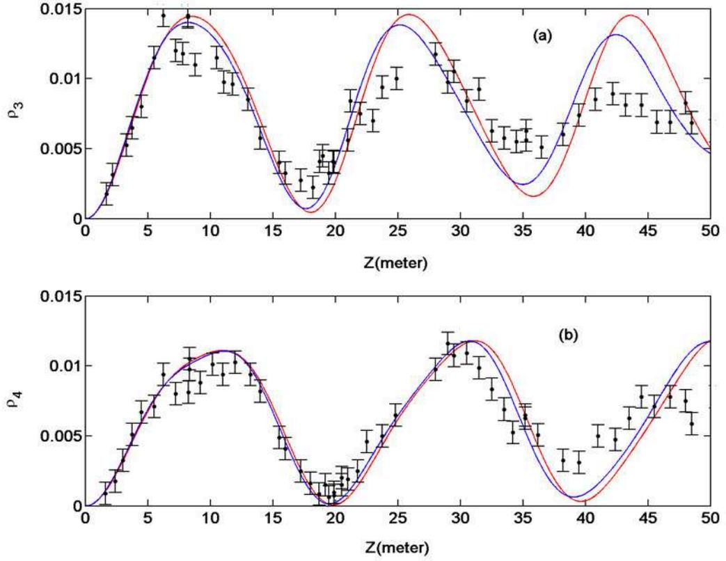
Figure A.4: Effects of inclusion of the pulsed nature (5 ns FWHM) of the input pump laser light on the first-order sideband evolution as a function of fiber length for  $P_0 = 2.1$  W. Dashed curves represent cw simulations and solid curves represent pulsed simulations.  $\Omega = 366$  GHz,  $\Delta\nu = 0.5$ ,  $\gamma = 0.019$  W<sup>-1</sup>m<sup>-1</sup>, and  $\beta^{(2)} = 55$  ps<sup>2</sup>/km (a) power in the blue-shifted sideband, (b) power in the red-shifted sideband.
