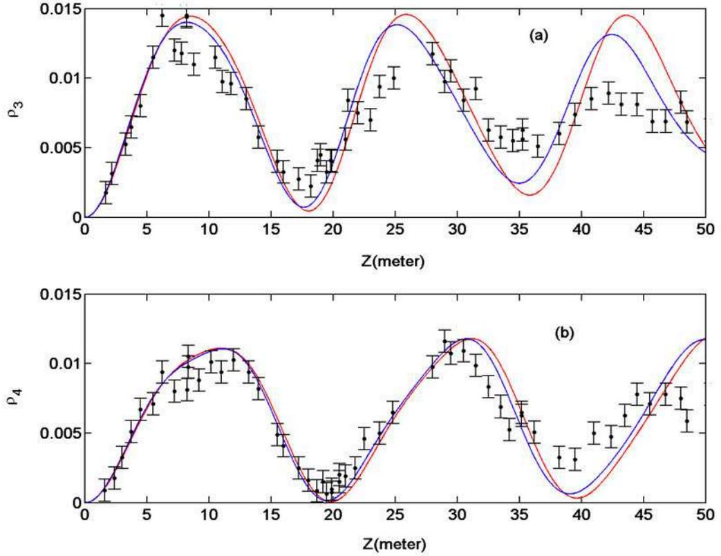
Figure 2.4: Effects of inclusion of the pulsed nature (5 ns FWHM) of the input pump laser light on the first-order sideband evolution as a function of fiber length for  $P_0 = 2.1$  W. Dashed curves represent cw simulations and solid curves represent pulsed simulations.  $\Omega = 366$  GHz,  $\Delta\nu = 0.5$ ,  $\gamma = 0.019$  W<sup>-1</sup>m<sup>-1</sup>, and  $\beta^{(2)} = 55$  ps<sup>2</sup>/km (a) power in the blue-shifted sideband, (b) power in the red-shifted sideband.
